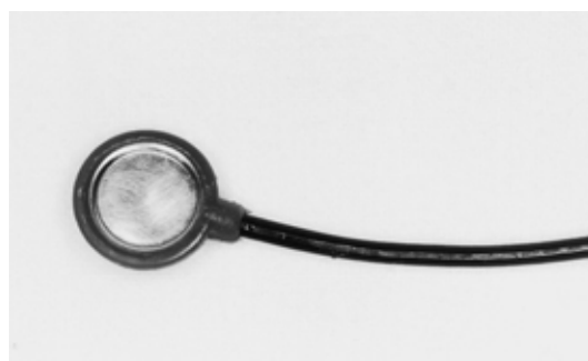
Fig. 1 A silver disc electrode of 8 mm in diameter for the measurement of sensory nerve activities
