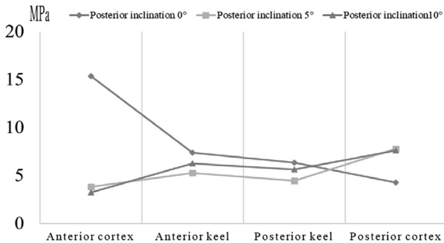
Fig. 4 Von Mises stress values for subchondral bone at the bone-implant interface (middle position; non-loosening model)
