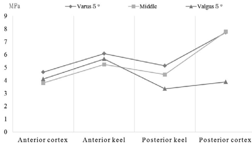
Fig. 3 Von Mises stress values for subchondral bone at the bone-implant interface (posterior inclination 5°; non-loosening model)
